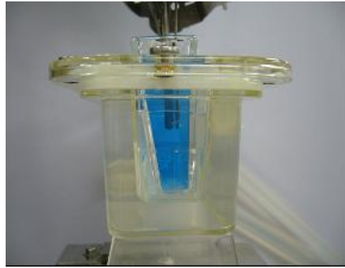
Fig.6 Side photograph: thermometer and vibrators in central unit
